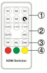
① IN1、IN2、IN3、IN4、IN5: Press this button will force switch the input port and the LED will indicate the corresponding input source. Note: IN4、IN5 in 3×1 Switch product is no function.
